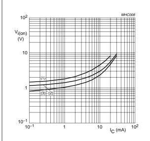
**TR1 (NPN);**  $V_{CE} = 0.3 \text{ V}.$
